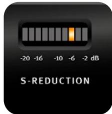
The S-Reduction LED display visualizes the intensity of the S-sound reduction between 0 dB and -20 dB in 2 dB steps.
