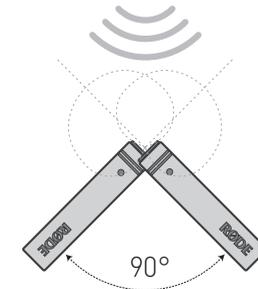
To mount your microphones in in X/Y configuration, follow the steps listed below. It's important to ensure that the microphones are placed at 90° to one another (right angle) with the capsules stacked above each other vertically.
