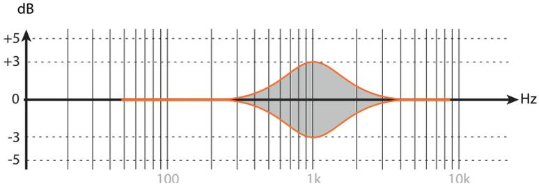
The Mid Filter is a bell filter with 1 kHz center frequency. It allows you to boost or cut the mid range up to +/-3 dB in 0.5 dB steps.
