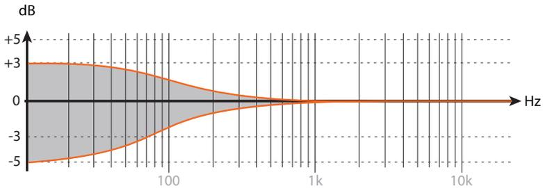
The Low-Shelf Filter allows you to boost or attenuate frequencies below 300 Hz in 0.5 dB steps. Use this filter whenever the acoustics of your room cause problems in the low frequency range.
