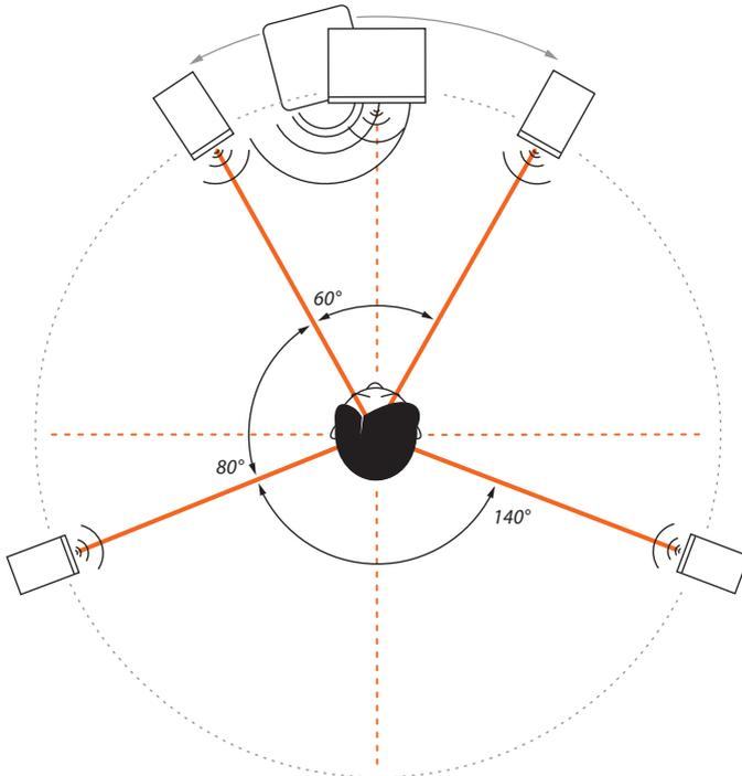
The rear satellites should form an isosceles triangle with the listening position forming an angle of 140°.
