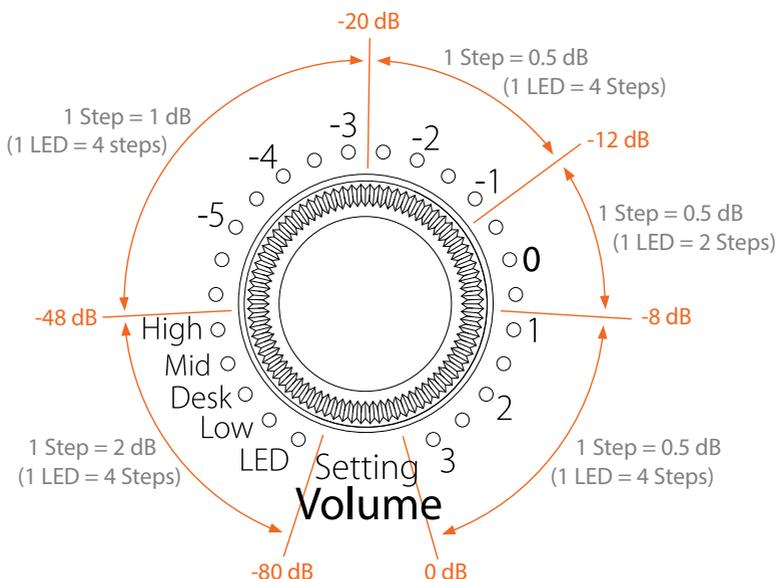
Turn the knob to adjust the volume. Depending on the LED mode selected (see LED mode), the volume will be displayed as a dim/bright circle or as a dim/bright point.
