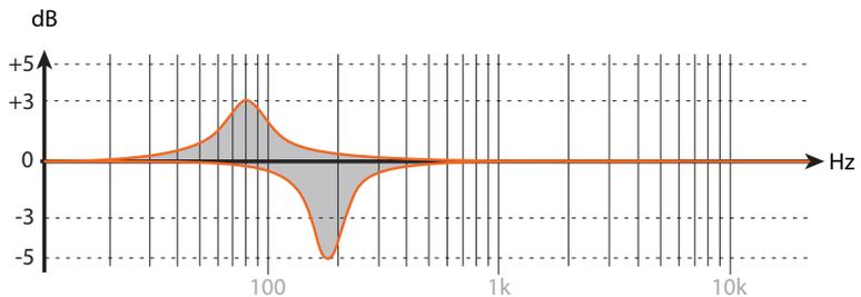
The Desk Filter has two functions. When turned down it acts as a narrow-band EQ set to 160 Hz (SC407 and SC408).
