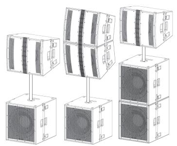
Ground-stacked, upward firing arrays, such as marching band applications that require covering the bleachers from a playing field are also supported. Up to (2) CDL12 loudspeakers can be mounted atop up to (2) CDL18s loudspeakers.
