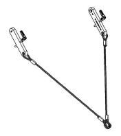
**CDL Rigging Sling**. The CDL Rigging Sling is required on all installations that include 4 or more CDL-series loudspeakers in a vertical array. Additionally, in installations using the CDL Rigging Extension Bar deployed with an upward or downward tilt of 12° or greater, the CDL Rigging Sling must be utilized.
