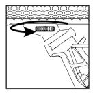
1. To relocate the handle, first turn the handle locking dial to the left several times to loosen the handle.
