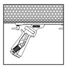
3. In addition to moving along the rail, the handle can also be rotated 180° for greater flexibility of use.
