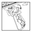
1. Open the 'quick release' angle clamp on the left hand side of the handle, and move the handle to the desired angle.
