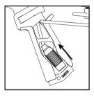
3. Remove the XLR cable from the handle by sliding upwards then through the handle as necessary to release the cable.
