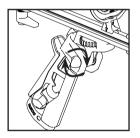
2. Tighten the angle clamp tension screw on the right hand side of the handle to increase the tension of the quick release clamp.
