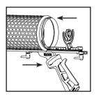
3. Slide the suspension body out of the main Blimp housing.
