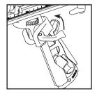
3. Close the angle clamp on the left hand side of the handle to lock it in place.
