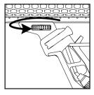
4. Turn the handle locking dial clockwise to tighten.
