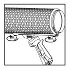
2. Loosen the front and rear rail clamping levers (approximately 1-2 turns).
