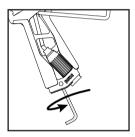
2. Using a 3mm hex key, unscrew the embedded XLR clamp/thread adapter, and remove it from the handle assembly.
