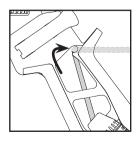
4. Secure the cable using the cable management clip at the top of the handle.
